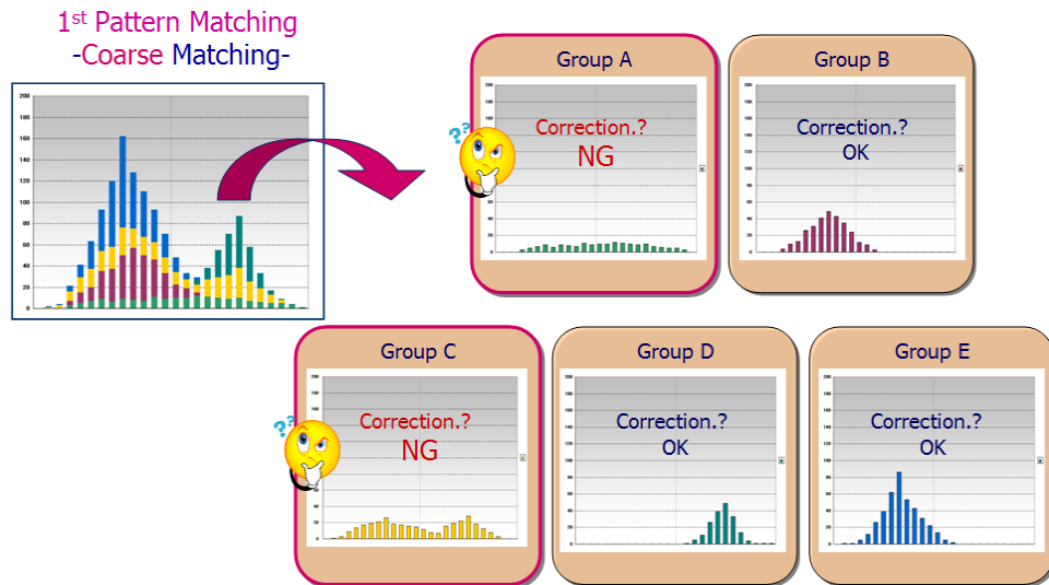
Figure 13. 1 st Pattern Matching – Coarse Matching
